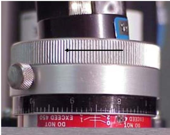
Each small mark on the dial is 1/10 microliter, each large mark is a one microliter change in the output of the pump (per 1 revolution). The pump is revolving at 3400 RPM. At the speed the oil head is traveling across the transfer roller, the pump actually revolves about 2-1/2 revolutions as it crosses one board.
